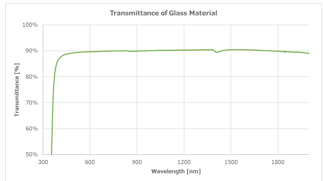
Figure 8 : Transmission vs. Wavelength (for 5mm thickness)
