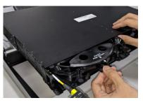
**5.1.3** Remove the protection tape, then start pulling out the cable up to desired length.
