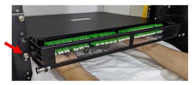
**4.2.2.3** Install additional screws on the mount bracket then tighten all the screws to secure the EVA panel in place.
