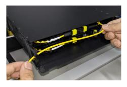
**5.1.8** Repeat the process for the other cassette, then after the procedure put the rear cover back in the chassis.
