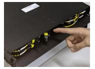
**5.1.2** Hold the pull tab of the MPO Adapter holder, then pull down to remove. Grope for the center guide lock, hold for it and swipe then pull out the spool cassette.
