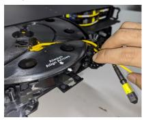
**5.1.5** Rotate the spool to align the arrows labelled on the top of the spool and cassette, then Push the lock to hold the spool and cable in place
