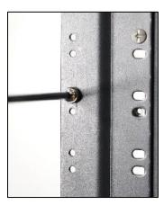
**4.1.2.2** Place the Spooling Patch Panel mounting brackets over the screws allowing the panel to rest on the screws.
