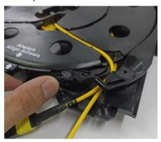
5.1.6 Partially return the cassette back into chassis, then get the MPO adapter holder w/ connected Fan-out and MPO Jumper inner end. Remove the Dust cap from the MPO Adapter and MPO Jumper Connector, then mate the Fan-out and MPO Jumper in the MPO adapter.
