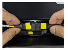
**5.1.7** Put back the MPO Adapter holder in the back of spool cassette. Hang the MPO cable in the rear cable hanger
