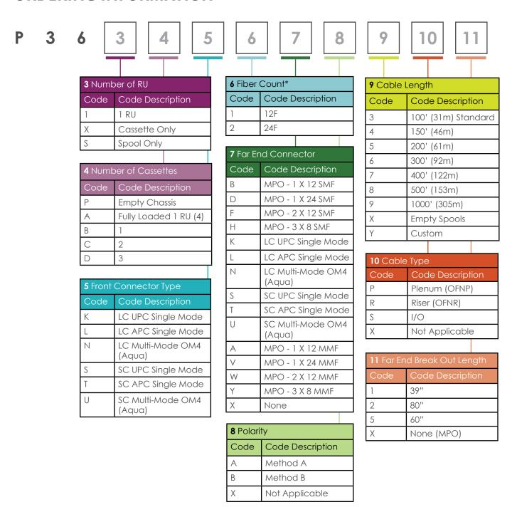
\*All cables are 3.0 mm diameter unless otherwise specified. Cable diameter affects the total cable length on spool.
