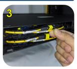
Grasp the pull tab of the MPO adapter holder and pull downward to remove it.
