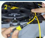
Route the Inner end MPO Cable from the top of the spool going out of the spool cassette
