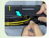
Push the rear lock sideway then pull out the spool cassette half way until the rear lock re-engage.
