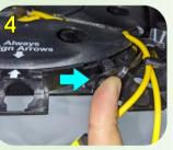
Push the lock until an audible sound "clicks" to hold the spool and cable in place
