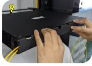
Repeat the process for the remaining cassette. Once completed, reattach the rear cover to the chassis.
