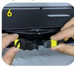
Retrieve the MPO adapter holder with the connected fan-out and the inner end of the MPO jumper.
