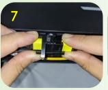
Connect the MPO to the Adapter, then reattach the MPO adapter holder to the rear of the spool cassette
