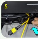
Partially insert the cassette back into the chassis
