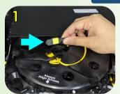
Take out the inner end MPO cable from the top of the spool
